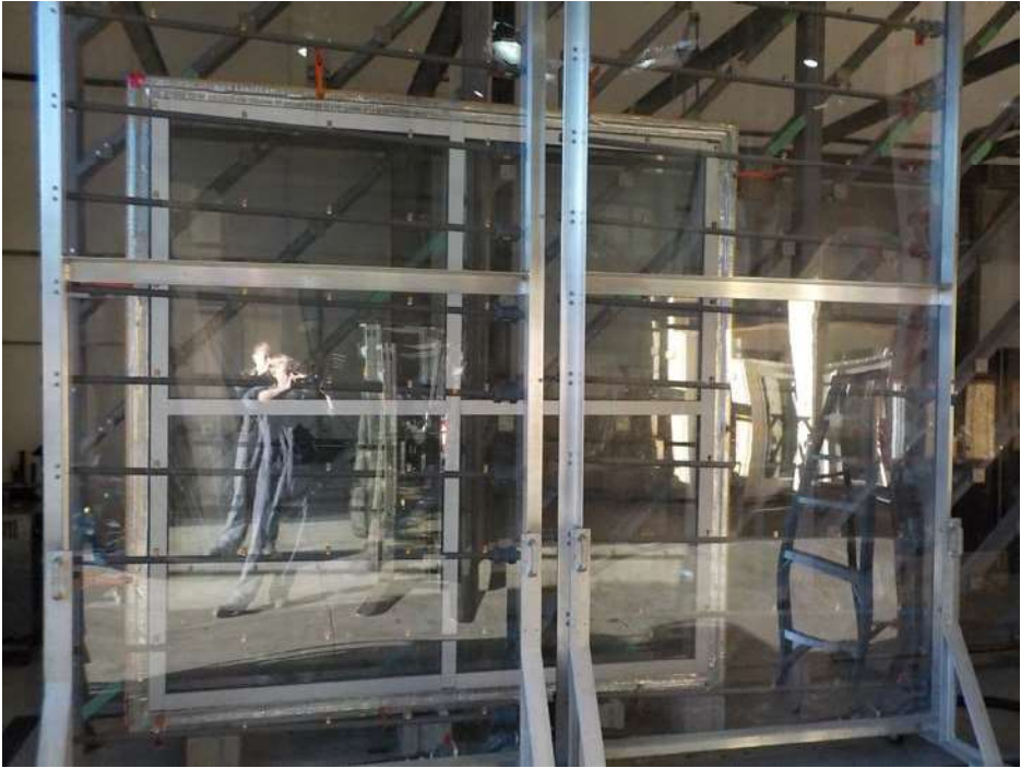
CW Series Multi-lite Fixed Combination Window – Water Penetration Test Set-up
