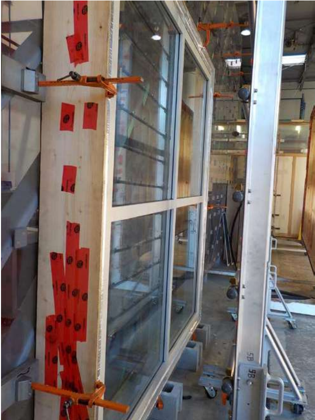
CW Series Multi-lite Fixed Combination Window – Water Penetration Test Set-up
